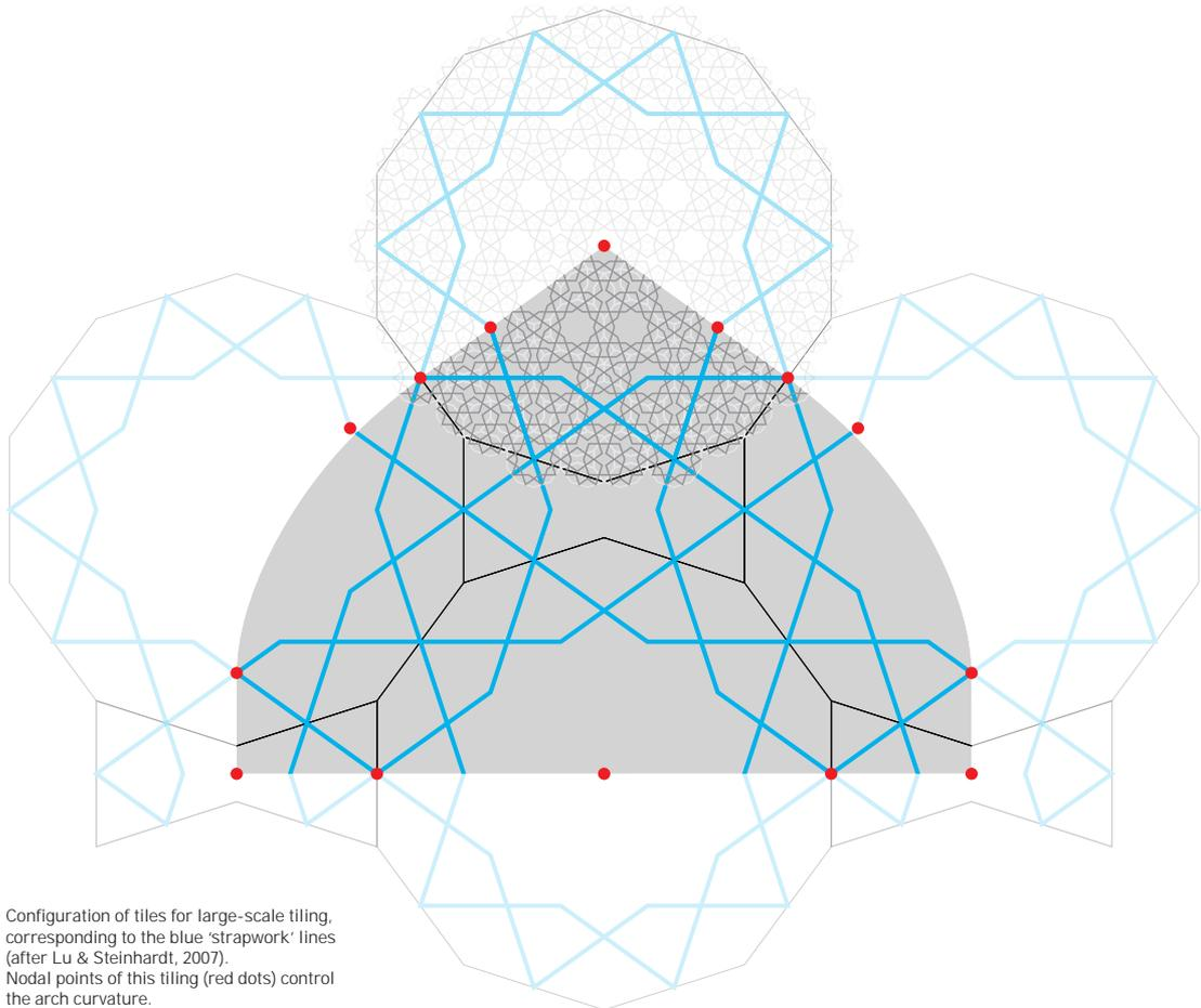
Configuration of tiles for large-scale tiling, corresponding to the blue 'strapwork' lines (after Lu & Steinhardt, 2007). Nodal points of this tiling (red dots) control the arch curvature.
