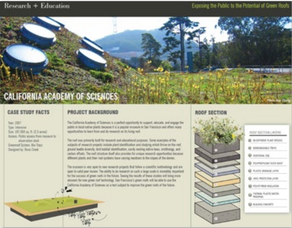
The California Academy of Sciences showcases the potential of living roofs in urban design. With over 1.7 million native plants, the roof provides habitat for local wildlife, improves stormwater management, and reduces energy use, setting a benchmark for sustainable architecture.
