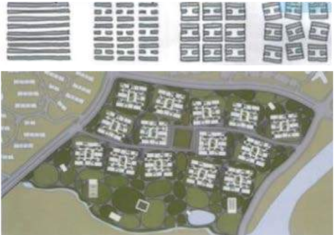
Figure 66: Diagram illustrating the morphology of one of the apartment complexes within Heronshire, a residential county. The individual blocks have been rotated and offset to increase the amount of interstitial landscaped zones between building blocks. Credit: Civitas
