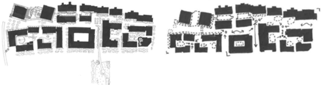
Figure 110: Building forms in Nadanohama complex and connection to green interstitial green spaces between buildings; (right) public spaces created off a main axis to form a pedestrian "mall" and intersection points
