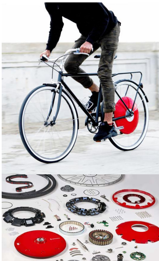
The 'Copenhagen Wheel' gathers data to learn how you pedal and ride and then automatically provides you with an extra boost when you need it.
