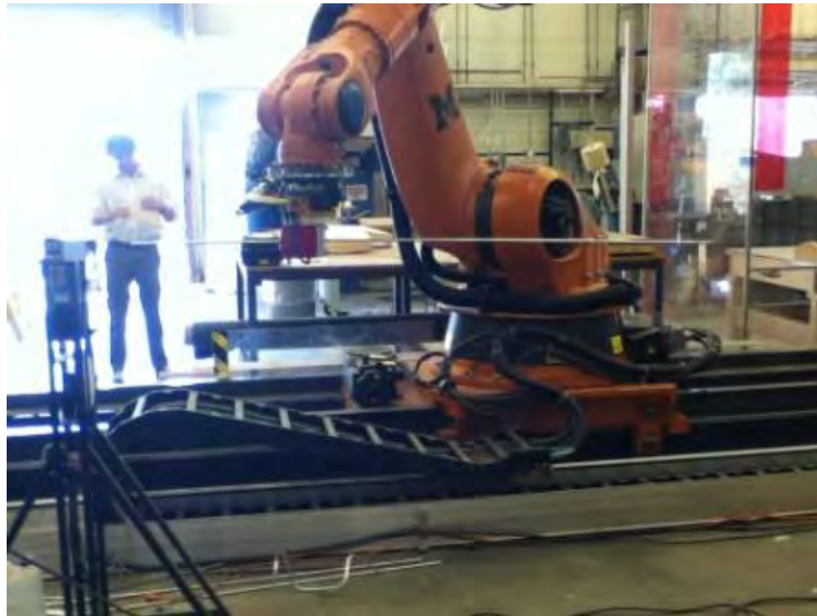
Robot undertaking digital rod bending fabrication
